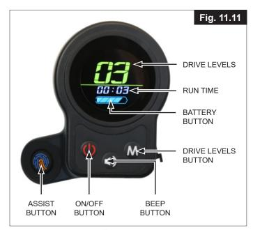
On/off method: press () short, beep once, to turn the R10 on successfully; press () long, beep once, to shut down the R10 completely.
