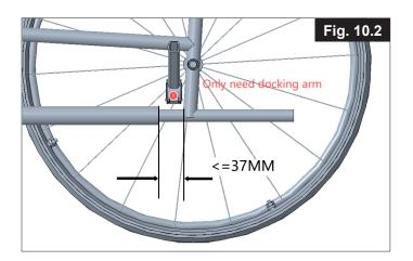
2. The limit block must be used, if the straight free space of circular tube for install docking arm is >37MM. (Fig. 10.3)
