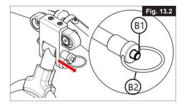
Step 4: Slide the rear control sequentially, remove it from the holder seat, and place the rear controller in the backpack.
