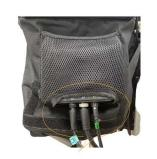
**Lithium Ion Battery**: the 5 Ah provides a range of up to 14km. It has a low weight and is easy removable.
